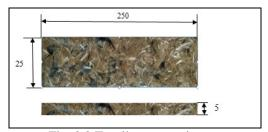
Fig. 3.2 Tensile test specimen
