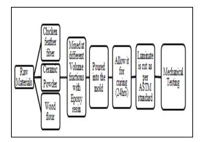
Fig 2.4 Hand Layup Process flow chart
